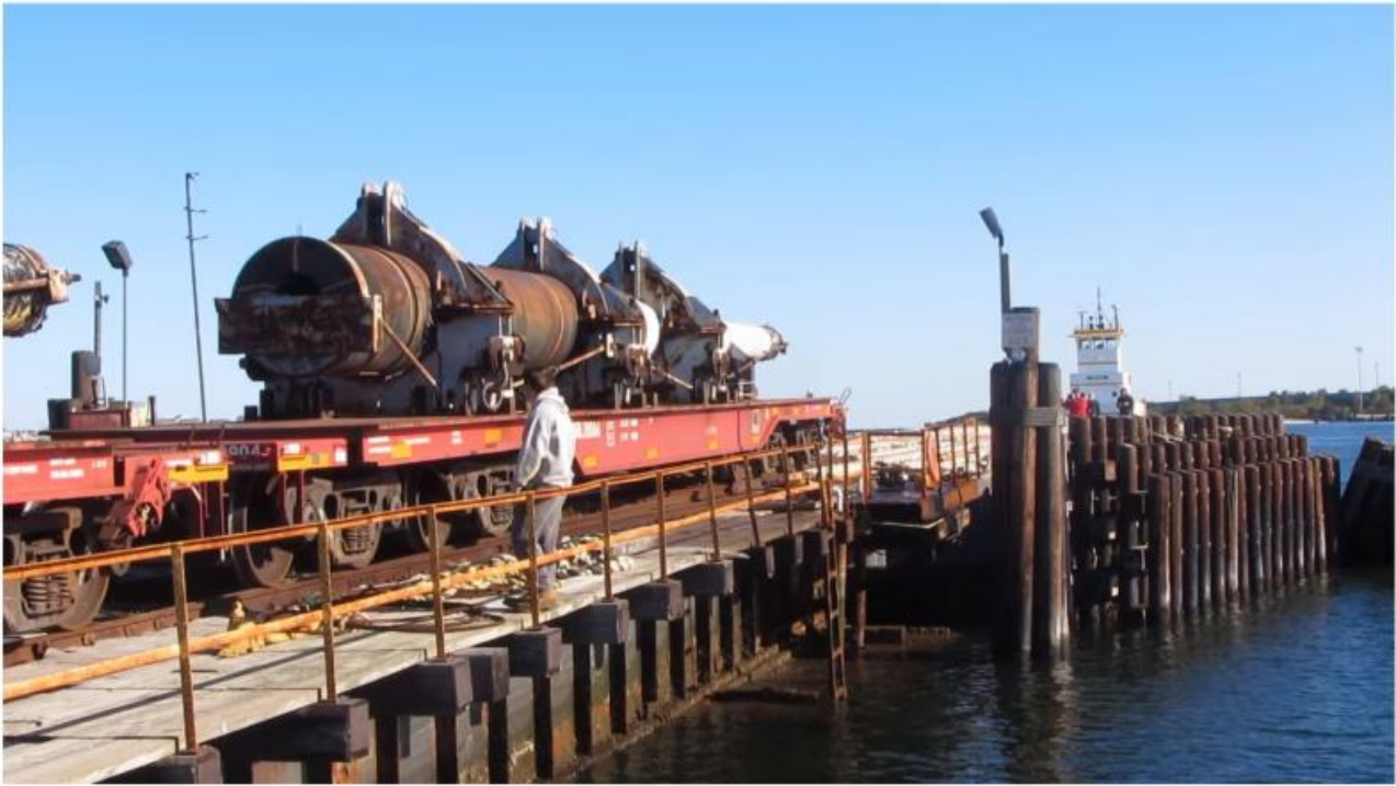
Eastern Shore - Bay Coast Railroad loading the battleship missouri gun barrels onto the carfloat
